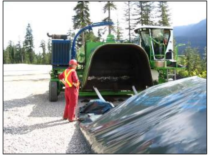
Raw compost is completely enclosed in AG-BAG eliminating leachate and odor issues. Compost under positive aeration. Temperature is monitored under OMRR regulation.
