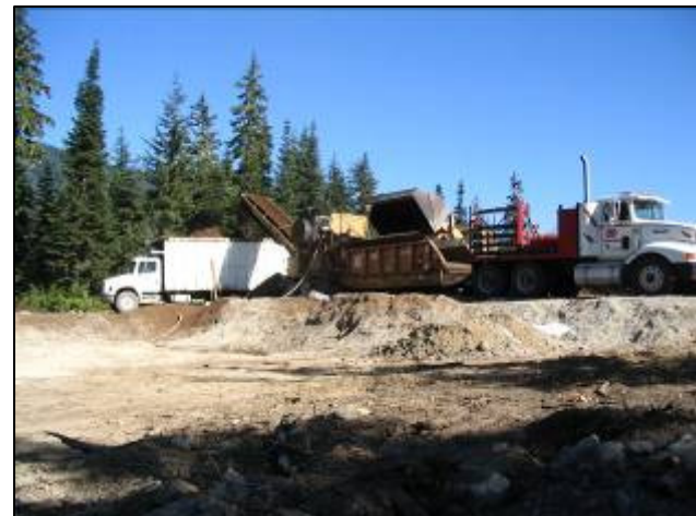
Mixing-grinding of wood waste (carbon) and nitrogen source prior to composting
