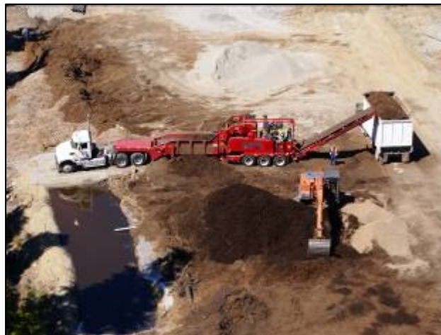
Mixing-grinding of wood waste (carbon) and nitrogen source prior to composting
